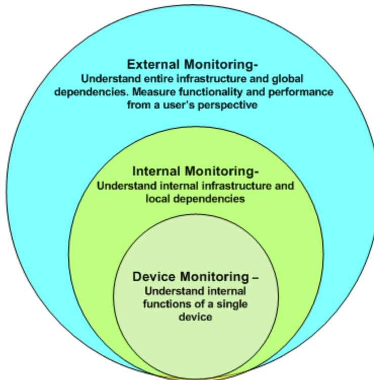
Figure 1.6: Different types of monitoring provide varying level of details with perspectives that range from device-specific to a global application experience.
