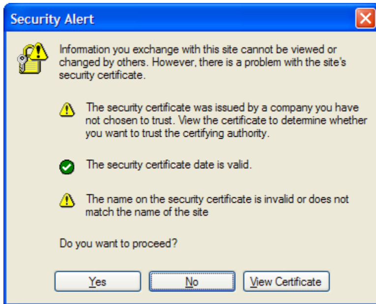
Figure 3.6: When a certificate is issued by an unknown certificate authority, an alert pops up.
