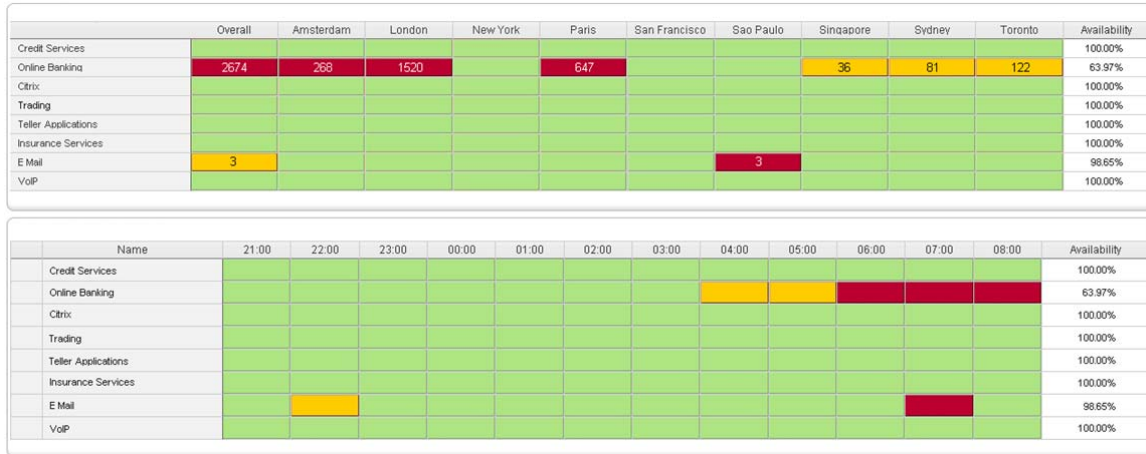
Figure 7.1: A top-level stoplight chart that alerts when systems violate established metrics for service quality.
