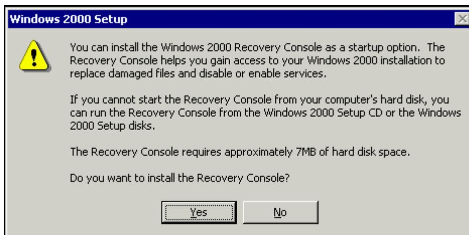
**Figure 2.14: Installing the Recovery Console.**
