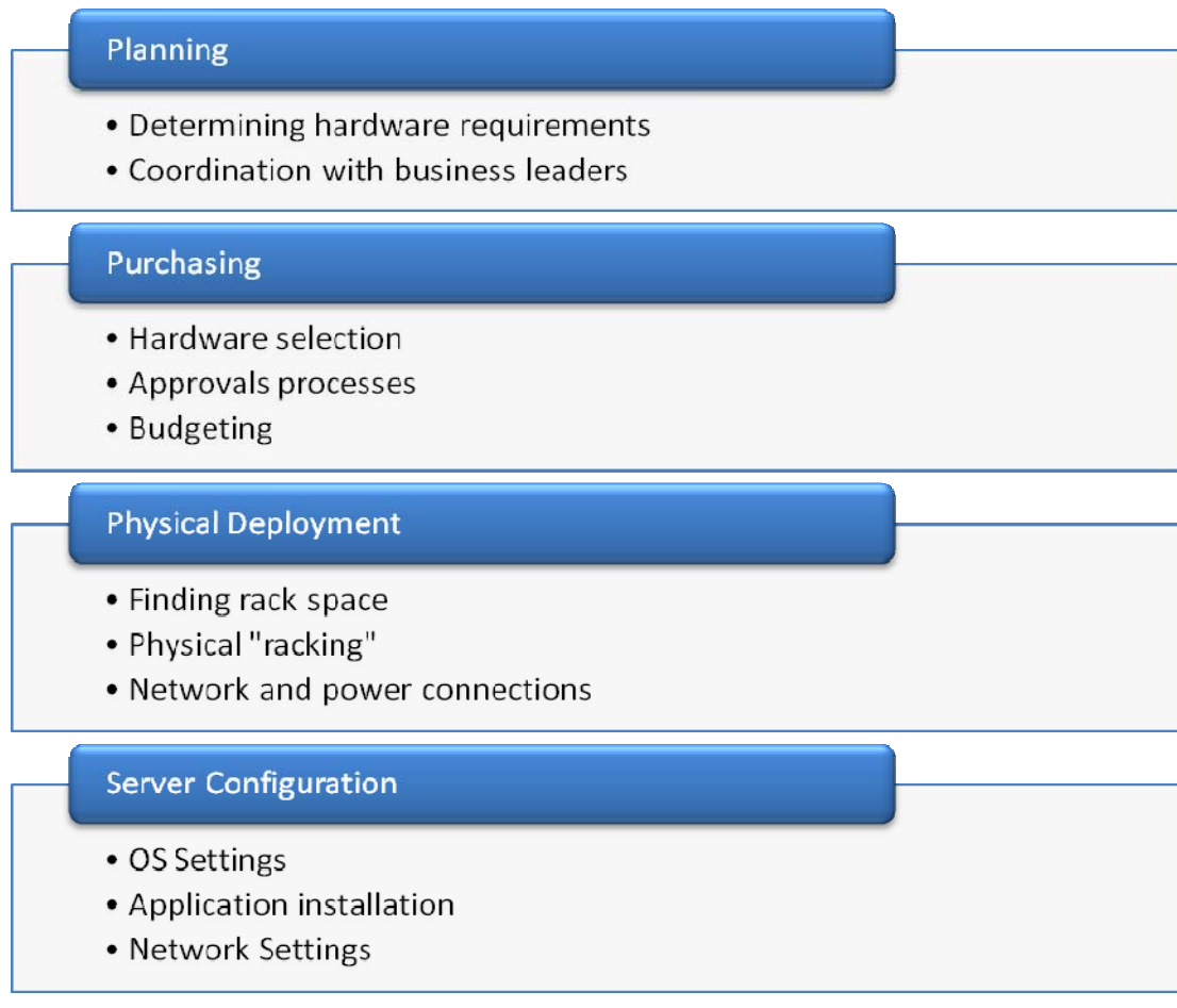
Figure 1.5: Steps involved in deploying a new server.
