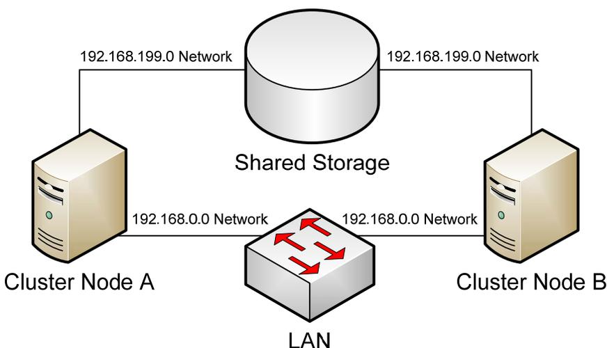
**Figure 10.4:** The networking configuration of our two-node cluster. This segregation of networks ensures that traffic routes through the correct network cards.
