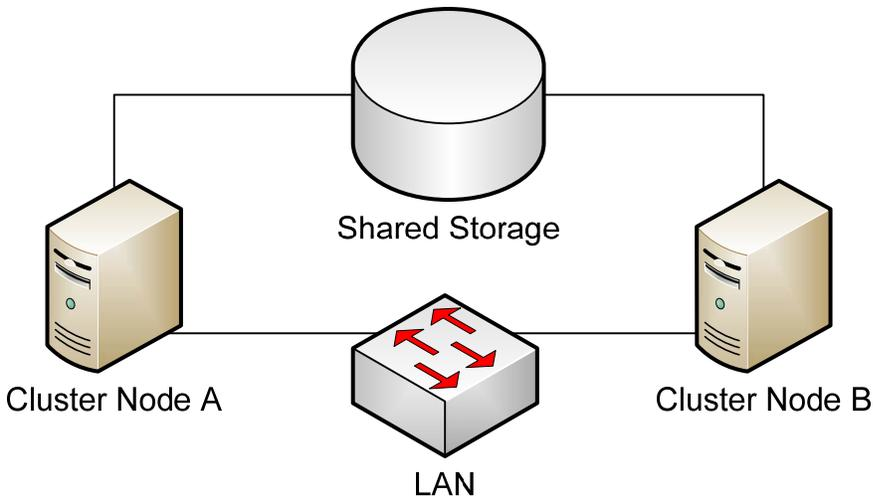
**Figure 10.1:** A high-level example of the resources used to build a simple two-node cluster.
