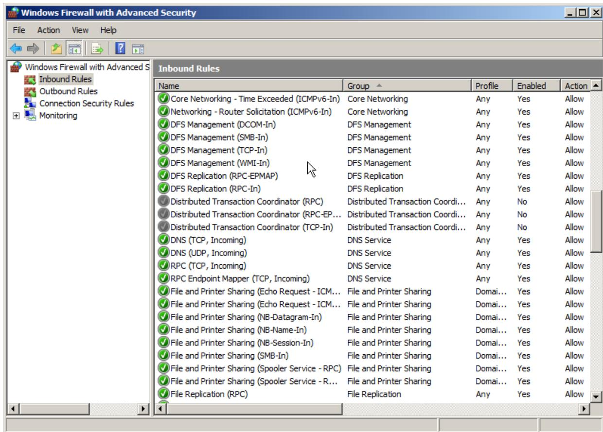
Figure 9.4: Inbound firewall rules displayed on an example server operating as a domain controller.
