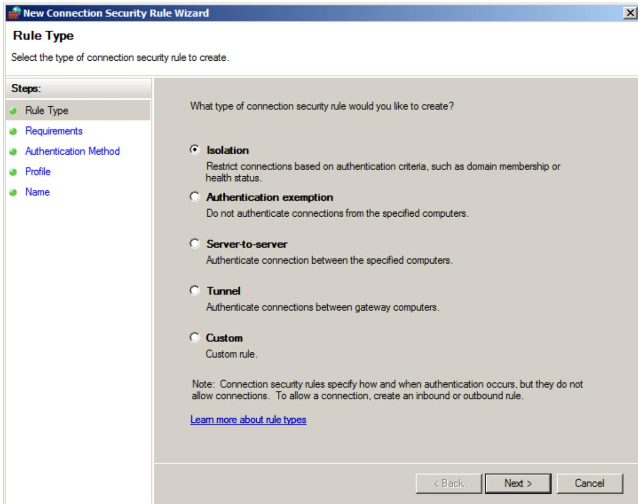
**Figure 9.6:** Connection security rules of various types are created through the New Connection Security Rule Wizard.
