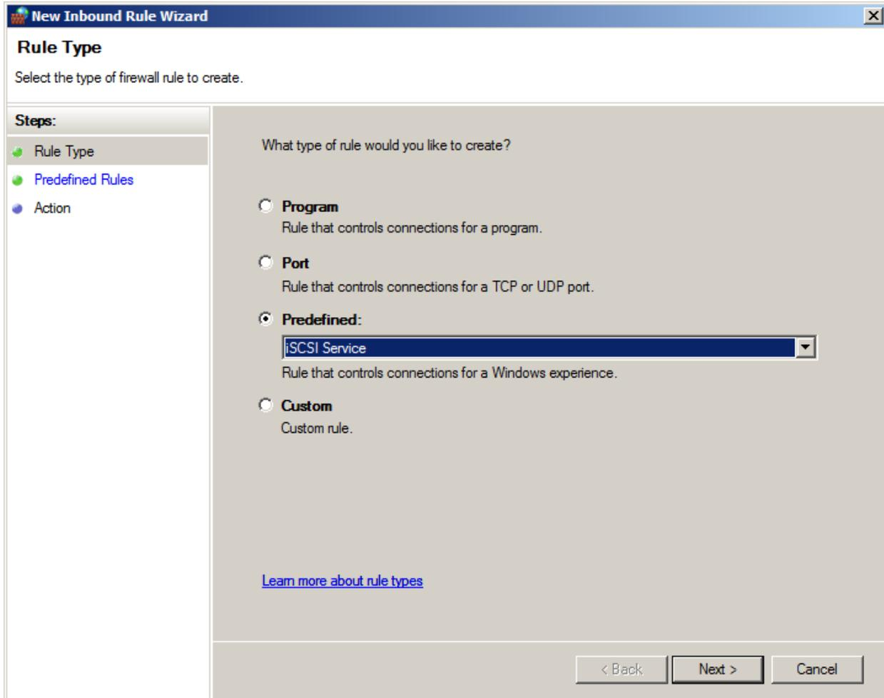
**Figure 9.5:** Configuring a new rule uses a wizard-like interface that enables rules based on actual ports, ports used by an installed application, or predefined Windows experiences.
