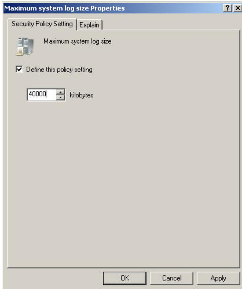
**Figure 6.3:** An individual setting within a GPO that configures the Event Log.
