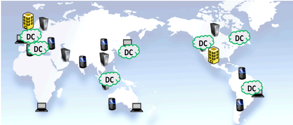
Figure 4.1: The implementation of multiple data centers offers a number of advantages, including resiliency to several potential problems (Image source: CDNetworks).
