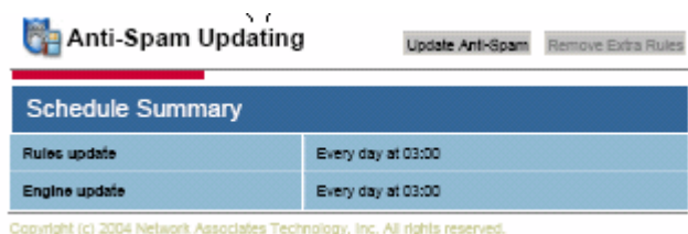
Figure 3.10: The automatic update facility allows for separate scheduling of signature file (rules) and scanner (engine) updates.
