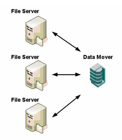
Figure 6.2: A server-less architecture relies upon the storage solution, or the components of its supporting infrastructure, to transfer the data.
