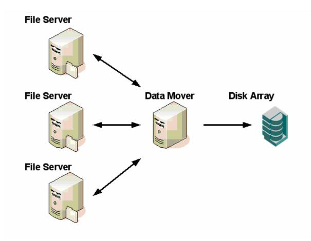
Figure 6.1: In a server-free design, a dedicated server acts as the data mover to free system resources on the target servers.
