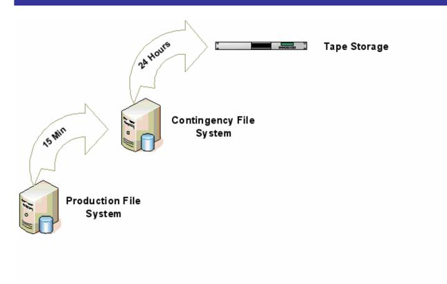
Figure 6.3: D2D2T and storage virtualization.
