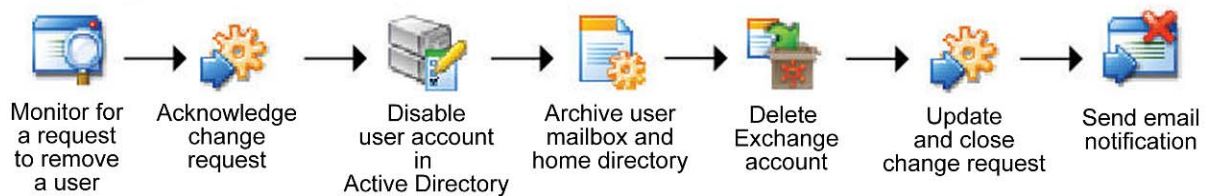
Figure 3.6: An ITPA security process for user removal.
