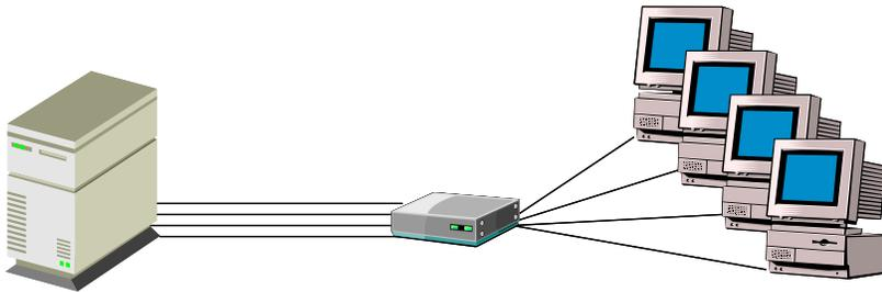
**Figure 2.5: Typical data transfer (individual streams to all systems).**
