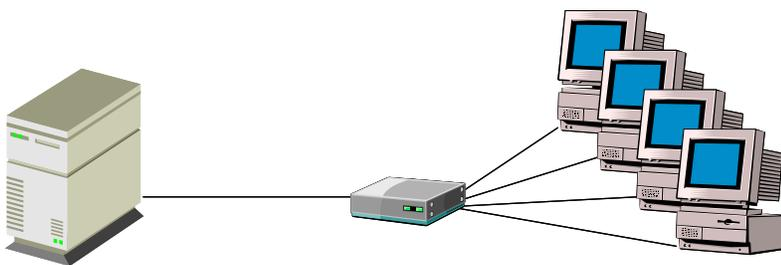
**Figure 2.6: Multicast data transfer (single stream to all systems).**
