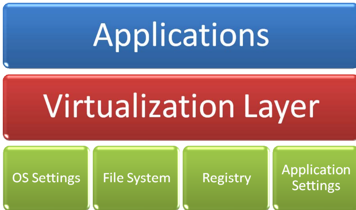
Figure 3.10: An overview of application-level virtualization.
