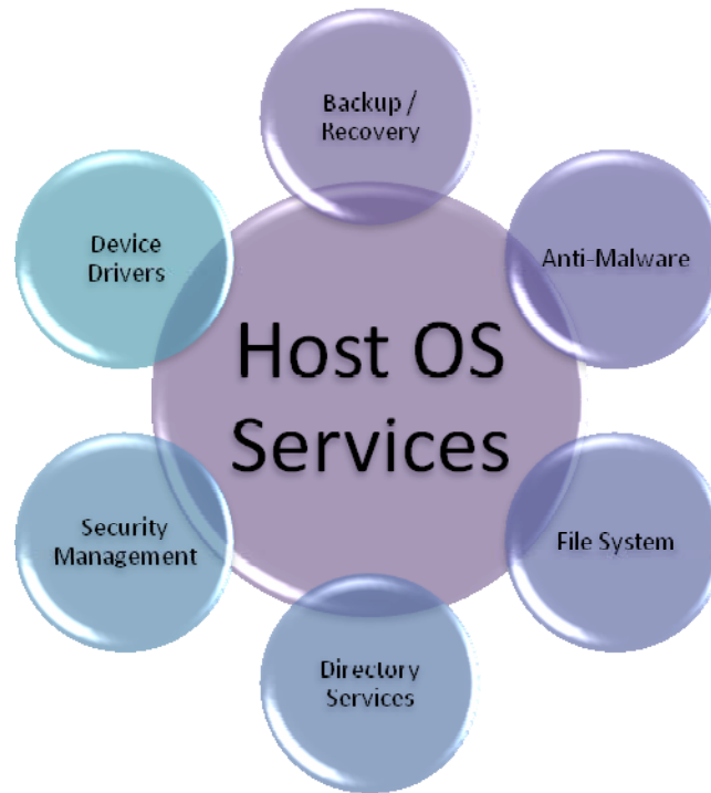
Figure 3.7: Host OS services and features that can be used by virtualization solutions.
