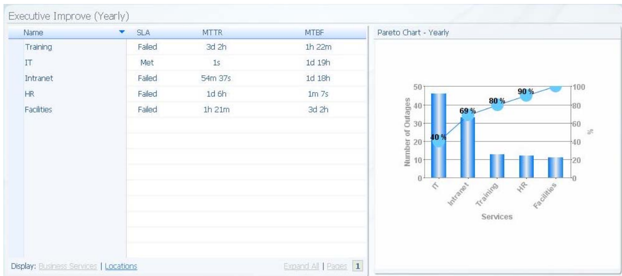
Figure 6.7: Dashboards can also be used to show the utility and failure rates of assets. This information provides insight into the need for future purchases or upgrades.
